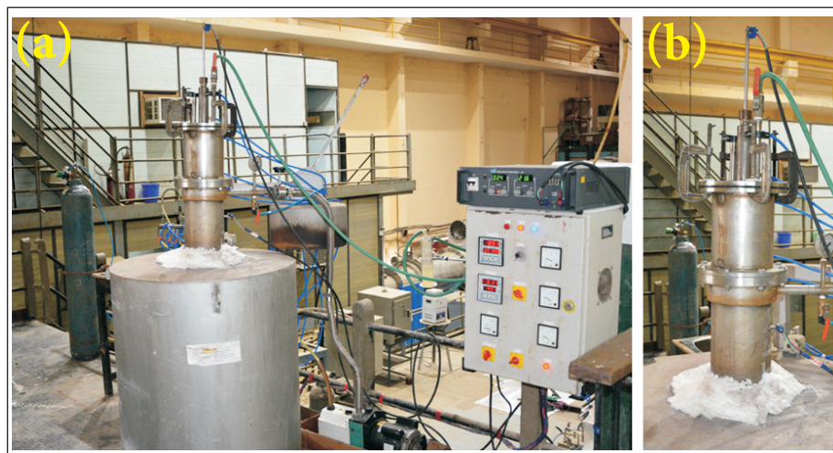
Fig. 1: (a) Molten salt electrolysis set up, and (b) Top part of the retort of the electrolytic cell
